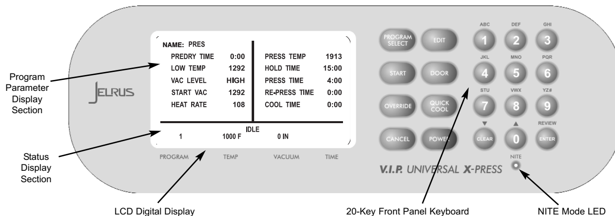
Figure 2. VIP Furnace Controls and Indicators Location
